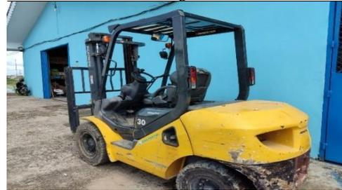
**Gambar 5.** *Counterbalance Forklift FD30-17 Komatsu*
